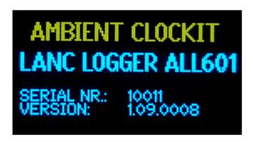
Press ESCape for 3 seconds, display will light up and show AMBIENT CLOCKIT LANC LOGGER ALL601 Serial Nr............, Software version........ After 5 seconds display changes to last selected job and settings with job open
