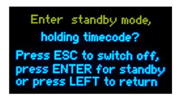
Press ESC for 3 seconds. Standby window will show Press ESC to switch off in 3 seconds
