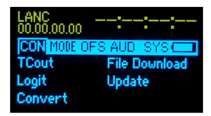
The JOB bar is configured to look like tabs in a filing system. On the right the battery capacity (Symbol) and System data menu (SYS) are displayed. On the left the job tab blinks,
