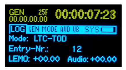
This job logs external timecode to internal TOD on a flash card and can also output TOD as Ext LTC with usebits containing cassette, event number etc
